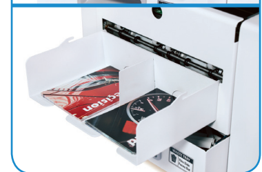
Adjustable catch tray keeps cards neatly stacked
